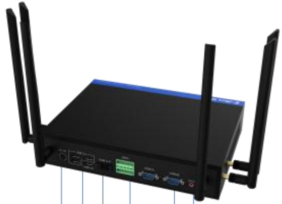
DC IN 4*USB 4*COM 16*GPIO 2*COM Mic & Line out
